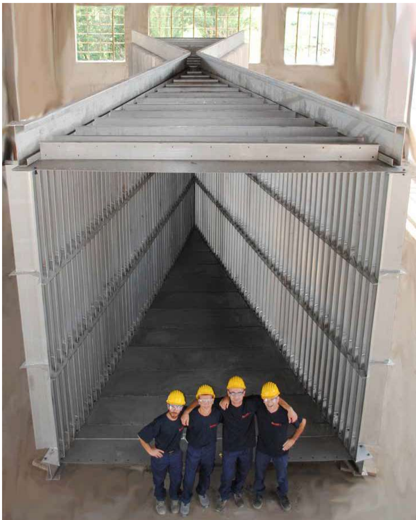
Vacuum Tower - Feed Inlet Vane Distributor Column diameter 16.000 mm - Nozzles diameter 3.600 mm
