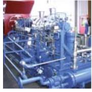
and expensive construction features. The GSG utilizes a full cartridge pullout design on sizes 100 and larger. A back-to-back option is also available.
