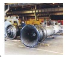
water lift, transfer and cooling water applications. A double suction variant, the BD, is available where NPSH is limited. When fitted with a can the BDC may also be used for condensate extraction applications. API 610 VSI, VS2, VS3 and VS6 versions are available.
