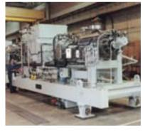
removal of the complete rotor for maintenance a simple procedure. They are particularly suited to low specific gravity applications where the back-to-back design and center bush provide natural axial balance and additional shaft support. These pumps also utilize the Sulzer Twistlock design for the casing cover.
