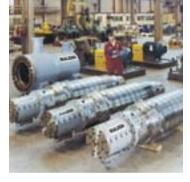
Using the Sulzer Twist-lock system of barrel closure to minimize weight, these pumps represent the state-of-the-art for upstream high-energy pumps. They are available in both horizontal and vertical configuration. The world's largest onshore, offshore, highest pressure and vertical injection pumps are all HPcp designs.
