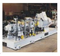
plications. Their design is optimized for synchronous speed direct drive applications thus avoiding unnecessary and expensive construction features. Their full cartridge design makes the most of the compact Sulzer Twistlock system of barrel closure. A back-to-back low flow high pressure option is also available.
