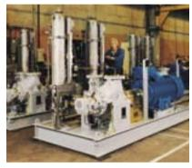
broad pressure and temperature capabilities of this design allow it to be used in the most arduous situations while still providing long and trouble free service. The double entry impeller is particularly suited to low NPSHA duties.
